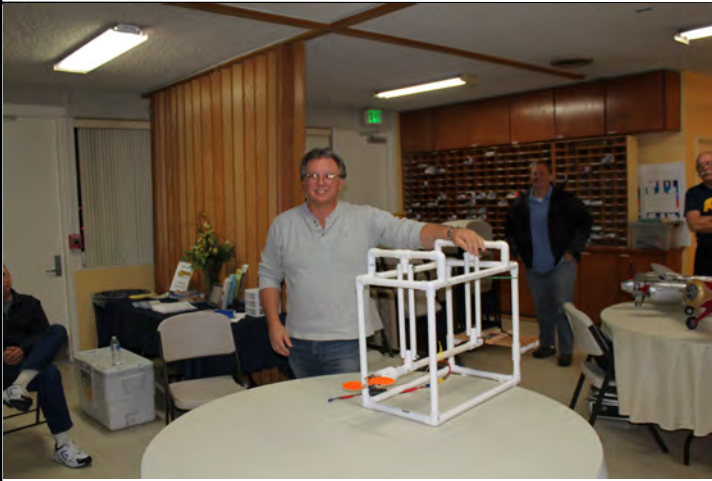
Rob Mawer designed and built this thrust Testing Platform.
